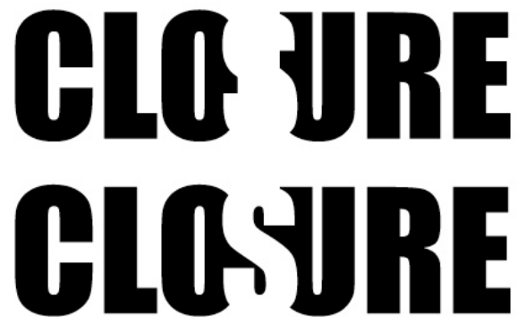
Fig. 5: Demonstration of the principle of closure. In the top example the closure is not enough to produce the closure effect immediately. Meanwhile in the bottom, there is more visual information about the missing part resulting in a higher accuracy but just enough so the user can complete the missing lines.
