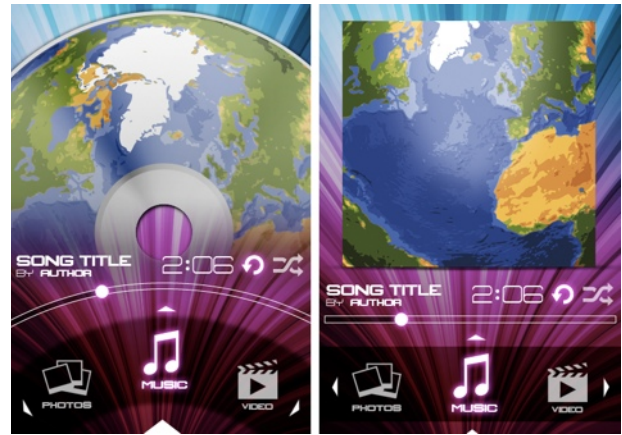
Fig. 12: Novelty is demonstrated in the left side of the figure. The interface displays a rotating interface rather than a flat one. Except for the song title group the whole interface is rotatory, even the timer bar. On the right side it is possible to see a demonstration of a traditional interface for music playing. It does display all the elements of the interface of the left but in a way that most music players in the market would display at the time of the writing of this research.
